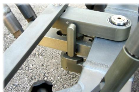
Switch lever (here in upward position)
