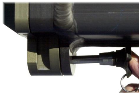
Securing the arm with a safety pin
