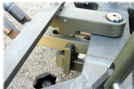
Switch lever (here in the downward position)
