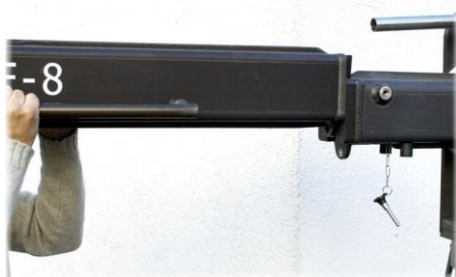
Mounting an extension arm
