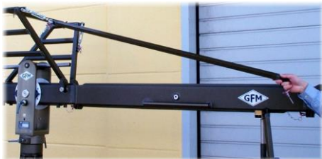
Connecting 1 x 142cm rigging rod to the turnbuckle
